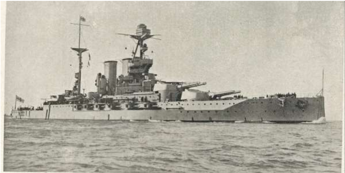
BRITAIN'S REPLY TO GERMAN NAVAL ESTIMATES: THE QUEEN ELIZABETH CLASS OF SUPER-DREADNOUGHTS The photograph shows Barham, fourth of the 13-inch gun battleships laid down in the Navy Estimates of 1912-13, and by which Britain again took the lead in armaments. Queen Elizabeth and Warspite were completed in October, 1914, and Valiant, Barham and Malaya early in 1915. These ships had a displacement of 27,500 tons; their length was 650 feet, beam 94 feet and draught 28 feet. Eight 13-inch and twelve 6-inch, together with twelve anti-aircraft 12-pounders, formed their armament. They were designed to develop 56,000 h.p., giving a speed of 25 knots, and had a 12-inch belt anti-ship. Each of these ships was built in two years, the same period as Colossus.
